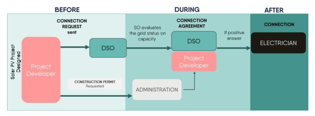
Grid connection procedure phases (simplified)
