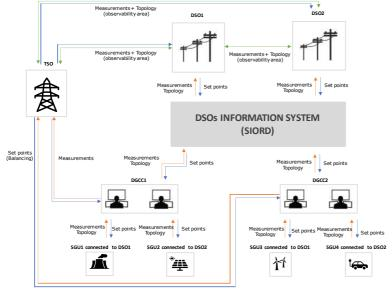
TSO: TransmissionSystemOperator DSO: DistributionSystemOperator SGU: SignificantGrid User DGCC: Demandand Generation
